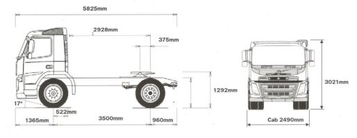
GVW : 21,500Kg GCW : 60,000Kg FRONT AXLE LOAD : 8,500Kg REAR AXLE LOAD : 13,000Kg
